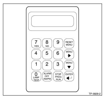
Figure 1-5 Digital Display and Keypad
